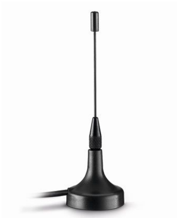
Figure 7: 868 MHz magnet foot antenna with 1.5 m antenna cable
